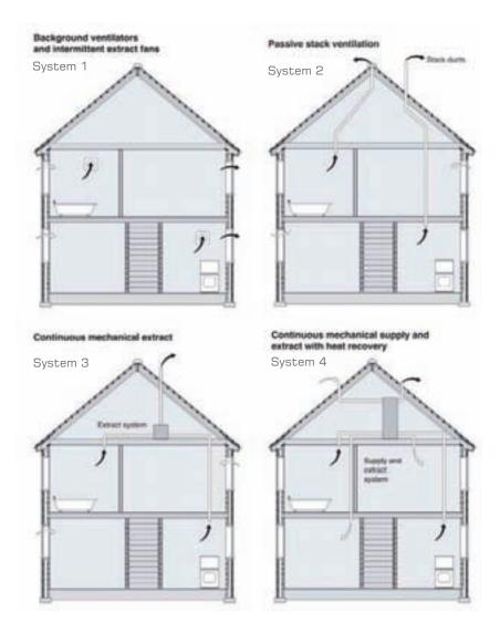
Figure 1 The four systems included in Diagram 2a from Approved Document F, 2010
