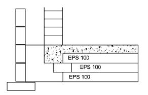
This is a variation of the above arrangement, with the addition of a small strip footing to support an external leaf of blockwork/brickwork. This strip footing should only carry the self-weight of the wall. Therefore all other loads such as roof and floor loads should be supported on the inner leaf, which sits on the ringbeam.
