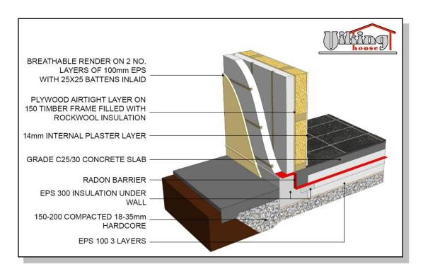
This arrangement is more like a raft slab and can be designed as such if required. The ringbeam and the floor slab are monolithic, with a thick EPS upstand at the outer edge of the ringbeam. This arrangement is suitable for superstructures with a large thickness of external insulation and also for ground conditions that dictate the need for a raft slab.
