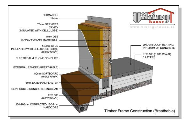
This is the most common arrangement of the Viking Insulated Foundations. The width of the ringbeam under the external wall can be varied to suit the dimensions and/or loads of the wall on top of it. The concrete ringbeam is tied to the floor slab through the EPS upstand to prevent torsion of the ringbeam, which could lead to uneven loading of the EPS 300 under the ringbeam with the associated uneven compression of the EPS.
