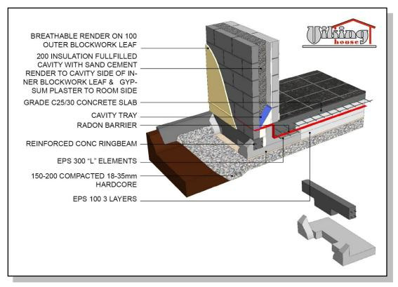
This arrangement is primarily designed to support a traditional blockwork cavity wall, but is also used for timber-frame structures with a masonry external leaf. The internal leaf, with floor and roof loads, is supported on a ringbeam at the edge of the slab. Appropriate reinforcement needs to be incorporated into the slab at this location.
