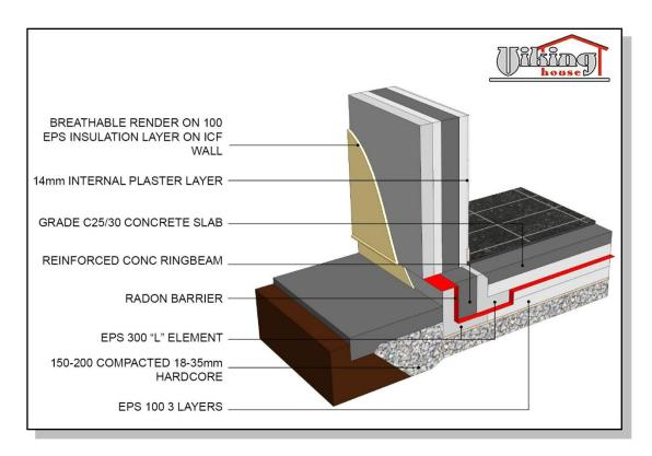
This is an almost identical detail to Arrangement No. 1. This detail is designed for an Insulated Concrete Formwork (ICF) superstructure.
