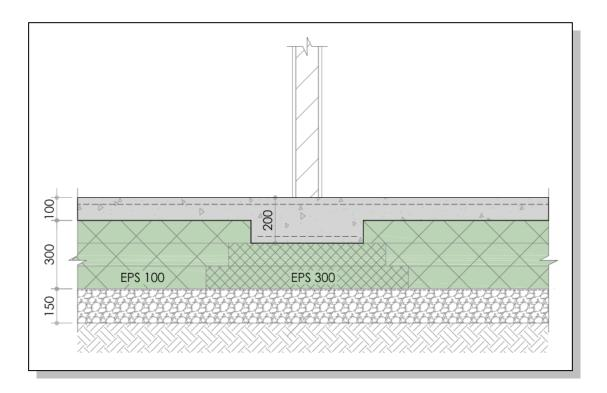
This is the typical arrangement for internal loadbearing walls. The width of the thickened portion of the floor slab can be adjusted to support larger line loads. The concrete needs to be suitably reinforced to adequately spread the load. The 2 no. layers of EPS 300 under the internal wall are made progressively wider than the thickening to allow the load to spread properly.
