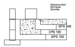
This arrangement is a further variation of the ringbeam with a widened base. This arrangement incorporates a separate strip footing to support an external leaf of blockwork/brickwork. The strip footing should support the blockwork/brickwork only and all other loads, such as roof and floor loads, should be supported by the inner leaf. Again, careful vibration of the concrete in the ringbeam is required to ensure the concrete extends fully into the 'toe'.
